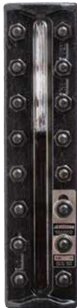
Reflex level gage showing about 60% oil
