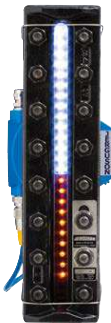
Transparent gage with illuminator showing 45% oil
