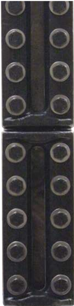
A Typical Dirty Glass Level Gage Without Illumination
